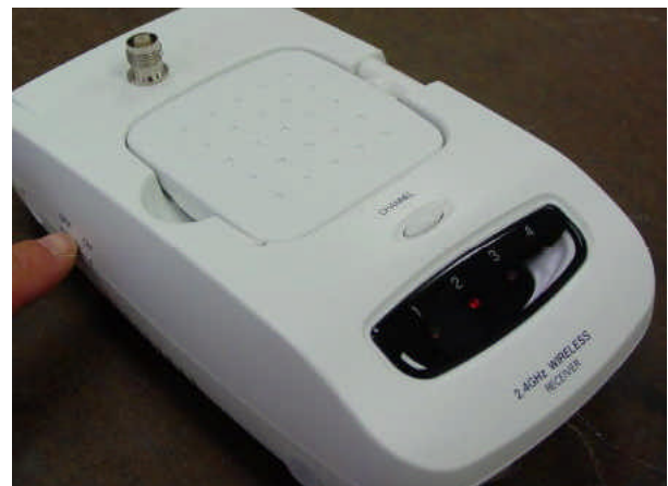
Figure 17. Receiver power & channel switches
