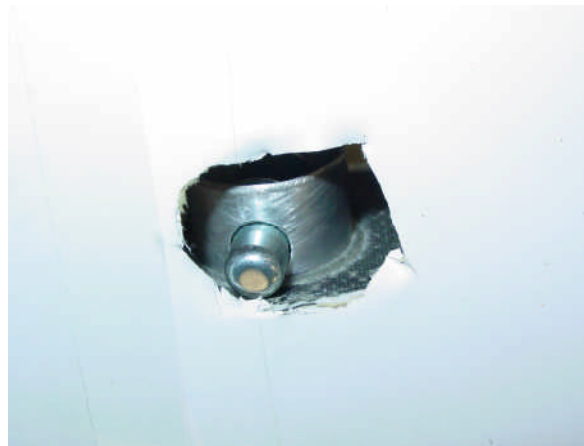
Figure 12. Wing spar snap-button locked in place
