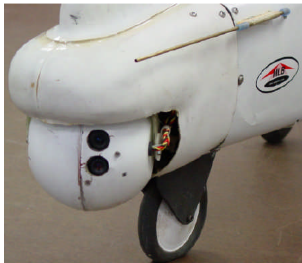
Figure 2. Nose assembly and airspeed probe
