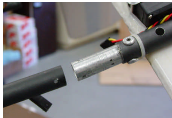
Figure 6. Tail boom & servo connections
