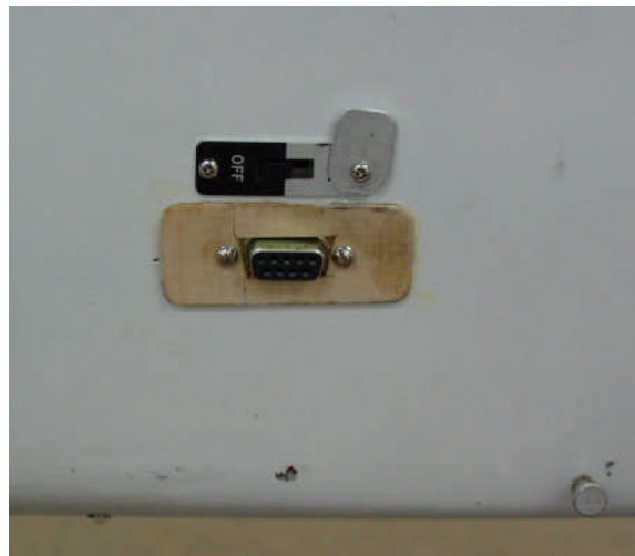
Figure 3. Power switch and serial port
