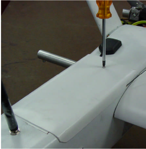
Figure 4. Access hatch screw
