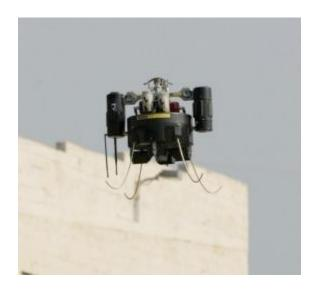
Air Vehicle is a packpackable ducted fan lift augmented Vertical Take Off and Landing Air Vehicle with gasoline powered engine
