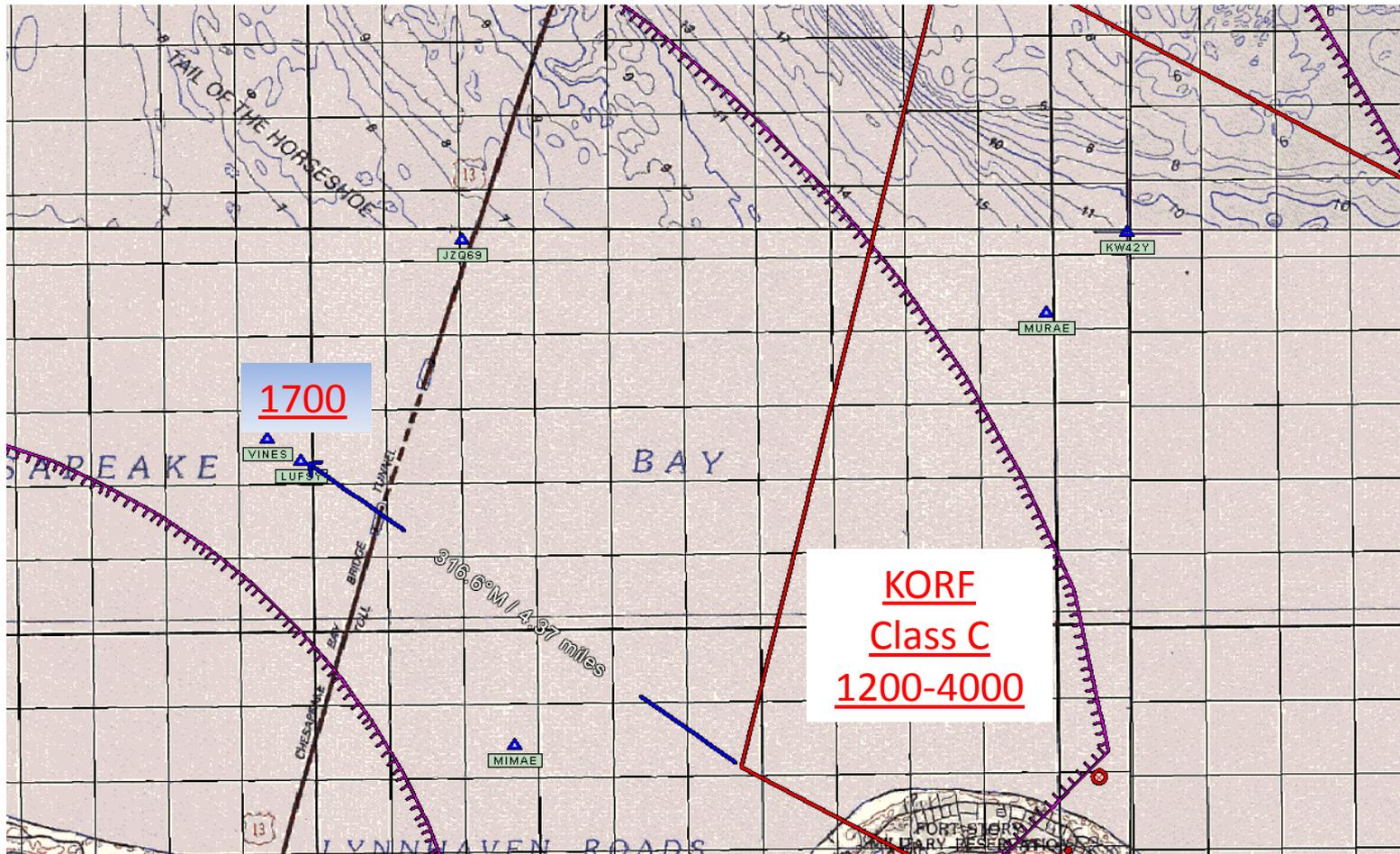
Lost-Data Link Recovery – Aircraft will descend below 500' AGL and proceed direct to the IP located N 36° 56' 00.50" W 076° 00' 15.03". The aircraft will cross the IP at or below 200' AGL and set up on a modified ¼ mile base, at or below 100' AGL, and align to the SkyHook. True Final Heading is determined with the last received wind data transmitted through the GCS.
