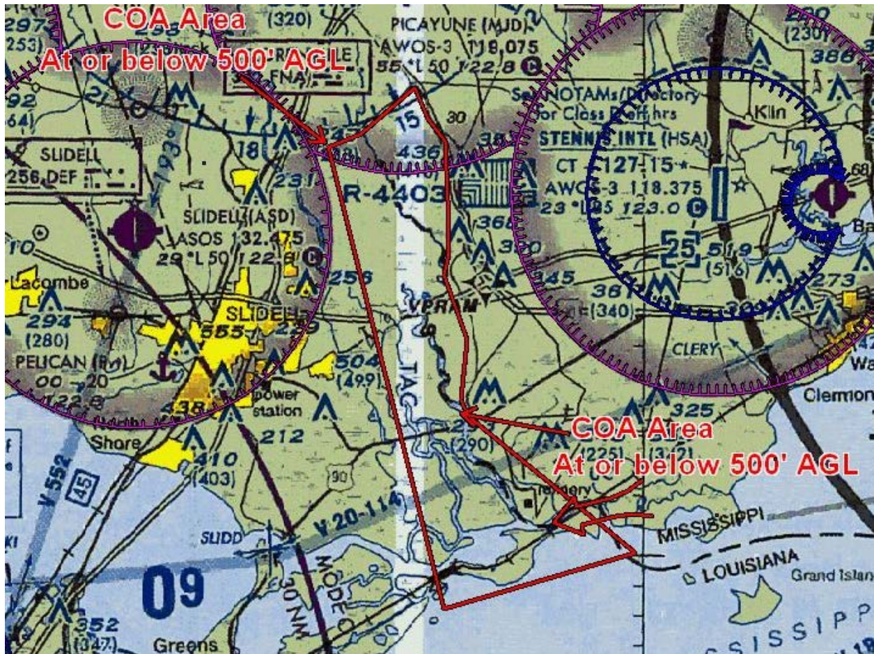
Figure 1. Wasp and Raven operation area / Stennis Buffer Zone / Class G Airspace Note: Altitude for Wasp is at or below 500 ft AGL. The Puma and Raven altitudes are at or below 1000 ft AGL except under the Picayune Class E airspace which the Puma and Raven will remain at or below 500 ft AGL.
