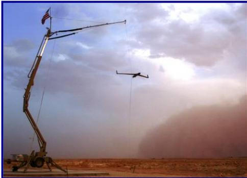
The patented SkyHook retrieval system captures the ScanEagle, providing near-vertical recovery on land or aboard a sea vessel. The SkyHook includes a GPS unit and antenna, which the UAV uses to make an extremely accurate approach, with precision measured in centimeters. The UAV is snagged on contact, by flying into the SkyHook rope, which is dangling approximately 50 feet above the surface. A hook on the UAV wingtip grabs the line and quickly stops the aircraft.
