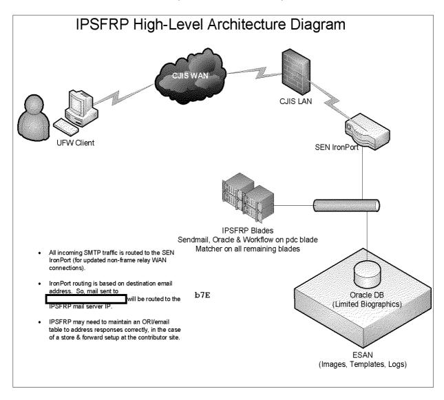
The IPSFRP system consists of 14 HS-22 Blades configured with 13 active Blades in an IBM Blade chassis with the additional blade serving as redundancy. Each blade provides computing services similar to a stand-alone server.
